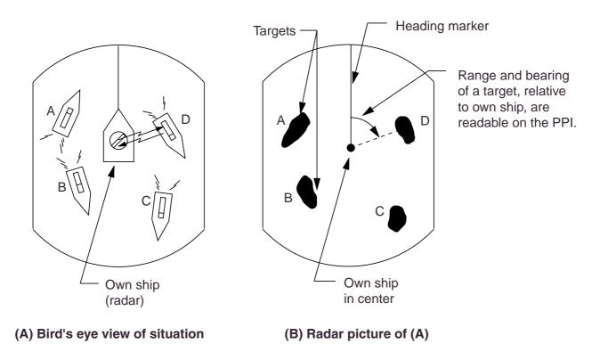
Figure 1-1 How radar works
